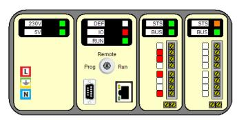
Parallel and serial links can work simultaneously, to allow fast exchanges (< 1ms) for some I/O and slowest
